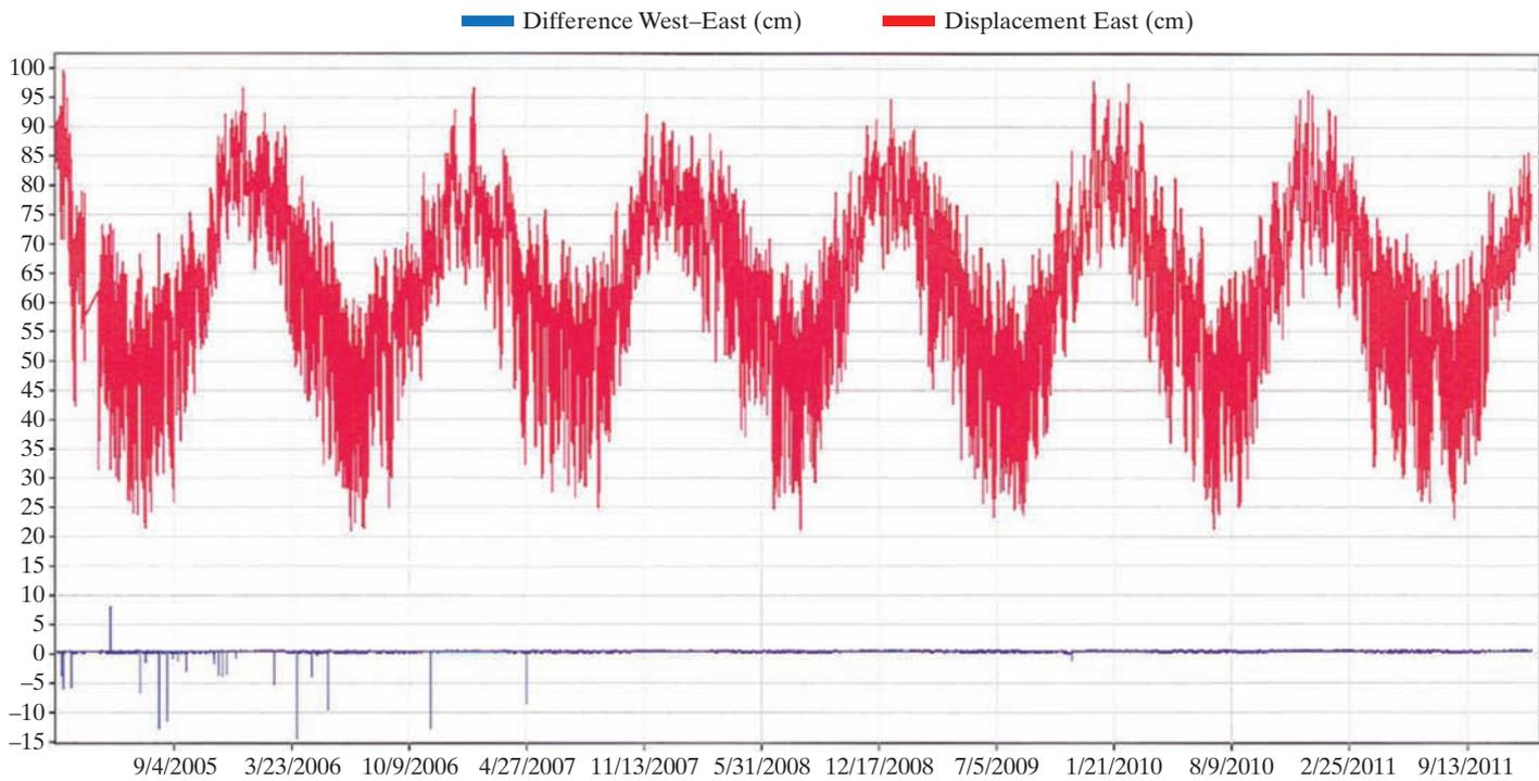
Fig. 7: Evolution of displacements at the abutment (Units y-axis: cm)
