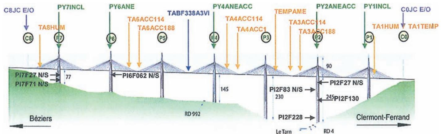
Fig. 4: System layout for viaduct instrumentation acquisition sets (Units: [-])
