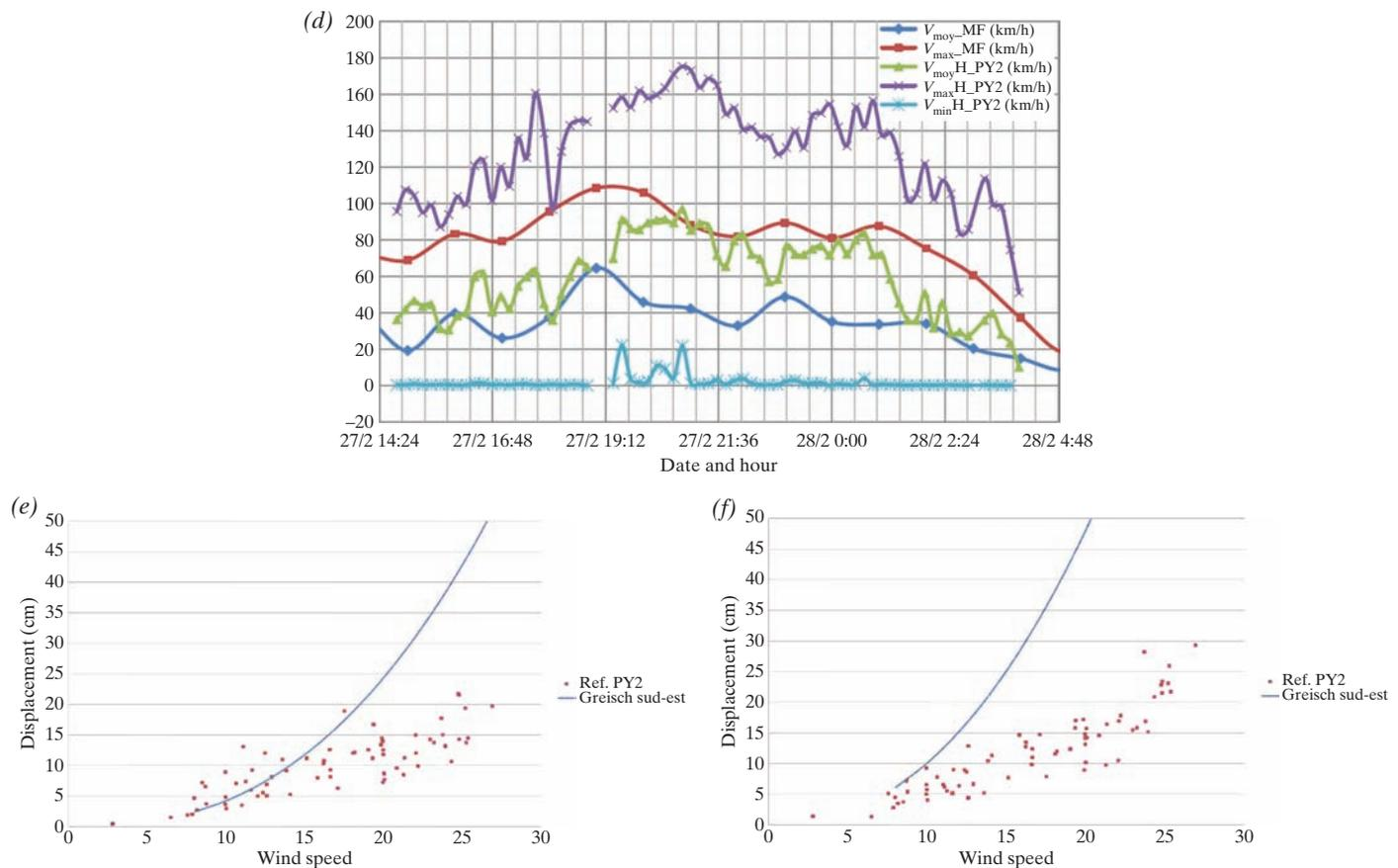
Fig. 8: Comparison of the different measurements and calculations during cyclones Klaus and Xynthia. (a) Cyclone Klaus, wind speed recordings; (b) transversal mode 1; (c) vertical mode 6; (d) wind speeds observed during cyclone Xynthia; (e) transversal mode 3 and (f) vertical mode 4 (Units Fig. 8e and f: y-axis: cm)
