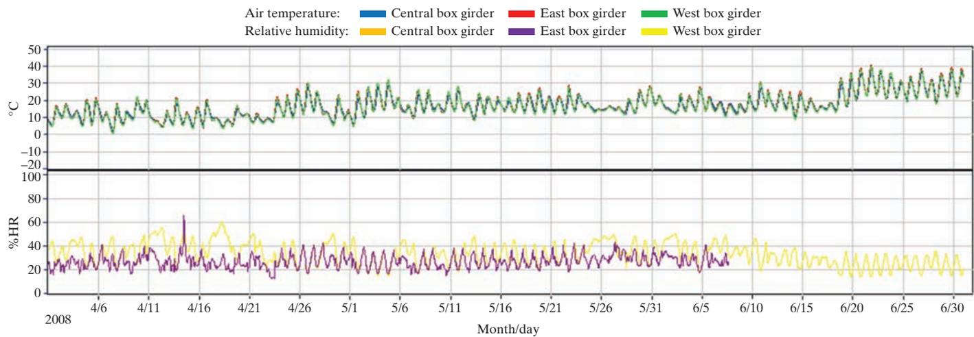
Fig. 5: Deck temperature and relative humidity
