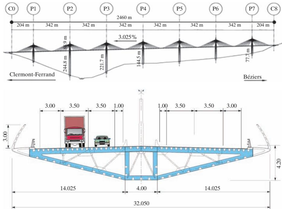
Fig. 2: Longitudinal view and cross-section of the viaduct
