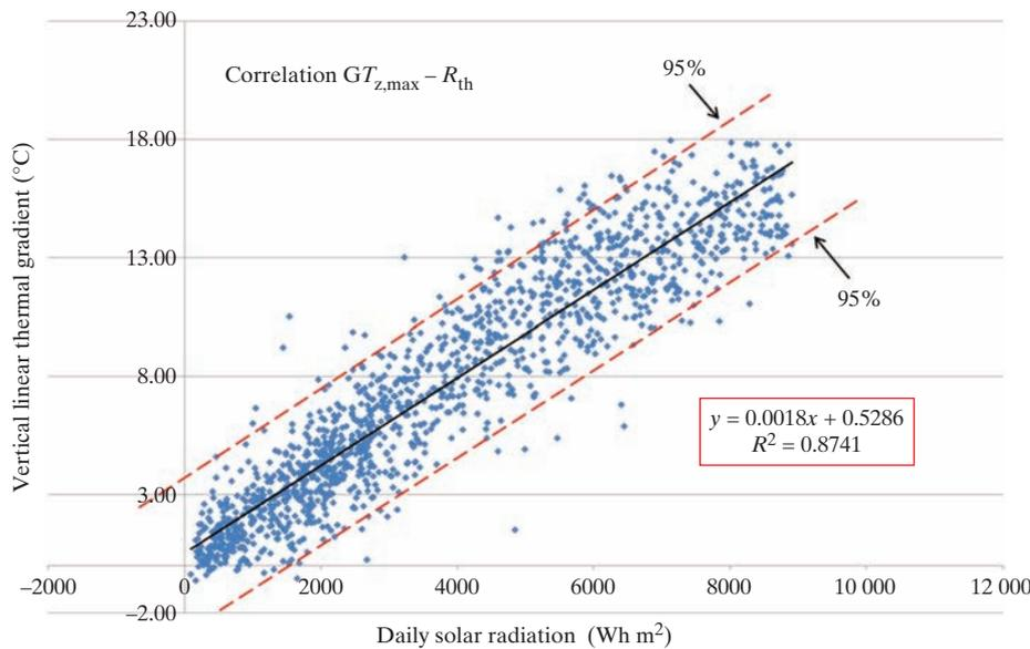
Fig. 10: Vertical linear thermal gradient according to daily solar radiation
